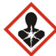
Severe health hazards
